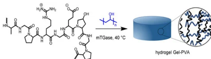
Fig 1. Pathway to prepare the Gel-PVA hydrogel. Microbial transglutaminase acts as a crosslinking agent.
