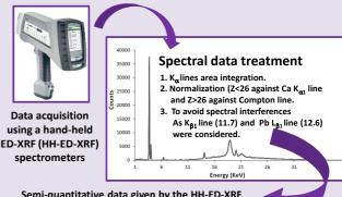
Semi-quantitative data given by the HH-ED-XRF instrument compared against a previously optimized WD-XRF method
