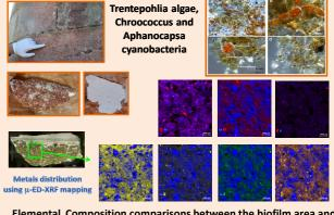
Elemental Composition comparisons between the biofilm area and unaffected building material using HH-ED-XRF methodology
