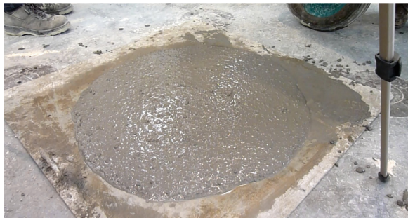
Fig. 1. Self-compacting concrete manufactured with EAF slag concrete
