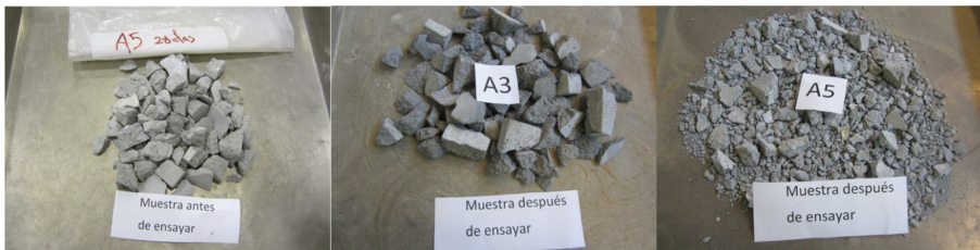
Fig. 3. a. (Sample A5 before testing); b (Sample A3 after testing); c (Sample A5 after testing).
