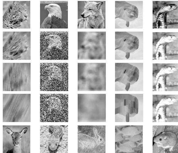
Figure 3.22: The exemplar input image patterns are shown in the 1st row. The 2nd through the 4th column below a given predator show the increase in the noise level or image corruption of the predator as discussed in the text. The bottom row illustrates the DLAM's recall performance when presented with a noisy predator image above the prey.
