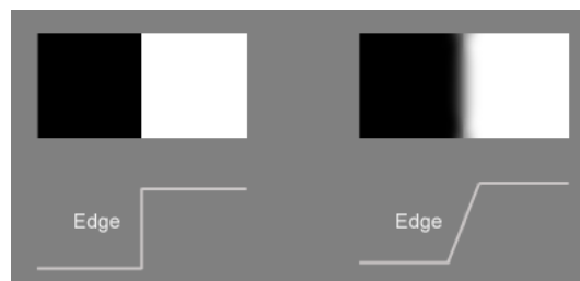
Figure A.9: (Left) Two surfaces ideally perfectly in focus, (Right) Soft boundary transition between two unfocused surfaces.
