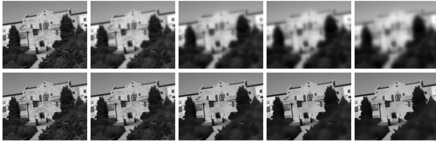
Figure 3.7: (Top) Linear Gaussian scale-space, (bottom) non-linear diffusion scale-space (image extracted from [5]).
